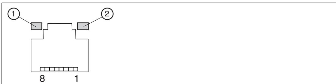
Figure 3.12 There are two LEDs next to the LAN port. The green LED ① is the Act/Link LED. The yellow LED ② is the Speed LED. Please refer to the table "LED display" below for the LAN port LED indications.
