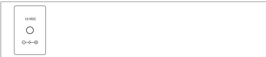
Figure 3.6 12 V<sub>DC</sub> barrel jack
