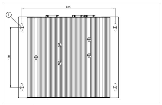
Figure 3.3 1 - for mounting screws Ø 5 mm
