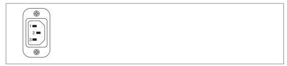
Figure 3.5 C14 receptacle 1 & 3 = AC power 2 = ground
