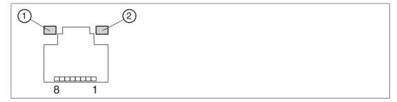
Figure 3.12 There are two LEDs next to the LAN port. The green LED 1 is the Act/Link LED. The yellow LED 2 is the Speed LED. Please refer to the table "LED display" below for the LAN port LED indications.
