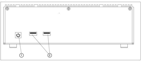
Figure 3.8 BTC01 Industrial Box Thin Client I/O Connection Ports, Front
