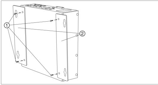
3. Use appropriate mounting screws with a diameter of 5 mm (not included) and the following mounting diagram to mount the unit to a wall.
