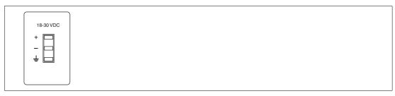
Figure 3.7 18  $V_{DC}$  ... 30  $V_{DC}$  terminal I/O plate
