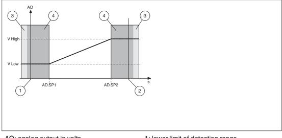
AO: analog output in volts V High: high voltage value V Low: low voltage value AD.SP1: position value setpoint 1 AD.SP2: position value setpoint 2
