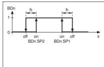
The output switches when an object is between SP1 and SP2.
