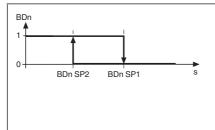
The output switches when the damping element falls below the SP2 position value and switches back when the damping element exceeds the SP1 position value.
