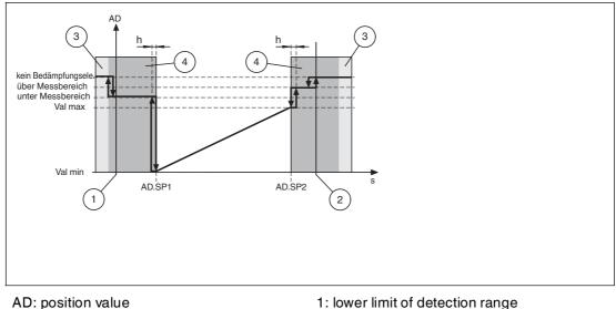
Val max: maximum position value Val min: minimum position value AD.SP1: position value setpoint 1 AD.SP2: position value setpoint 2 h: hysteresis
