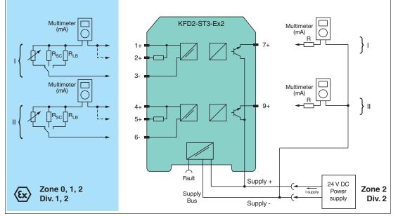
Figure 5.2 Proof test set-up for KFD2-ST3-Ex2
