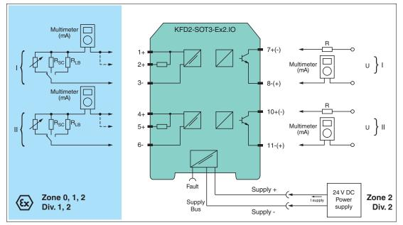
Figure 5.4 Proof test set-up for KFD2-SOT3-Ex2(.IO)(-Y1)
