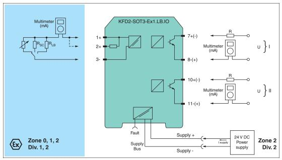
Figure 5.3 Proof test set-up for KFD2-SOT3-Ex1.LB(.IO)
