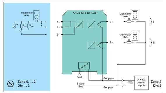
Figure 5.1 Proof test set-up for KFD2-ST3-Ex1.LB
