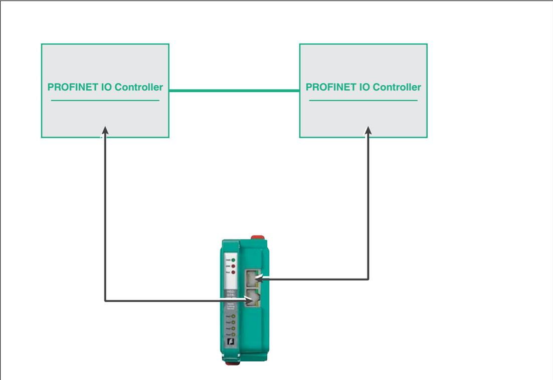
Figure 5.2 HD2-GTR-4PA.PN gateway in S2 redundancy according to the PROFINET specification
