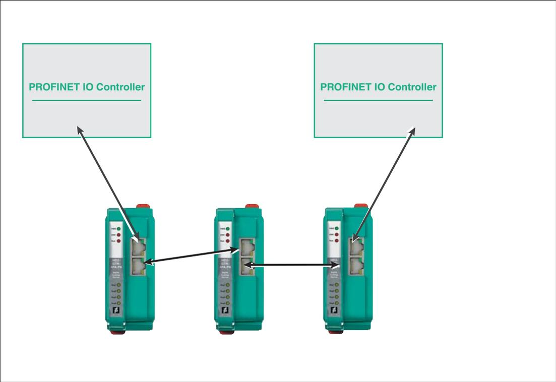
Figure 5.3 HD2-GTR-4PA.PN gateway in MRP ring redundancy according to the PROFINET specification
