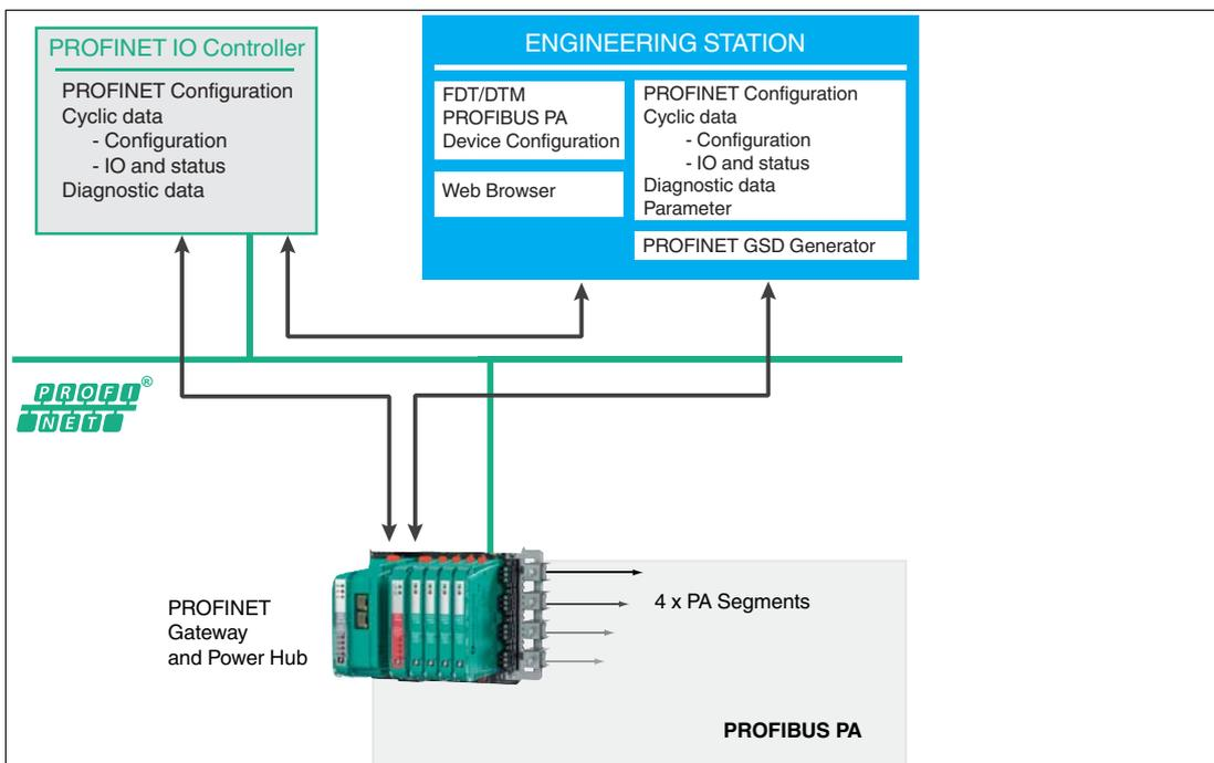
Figure 5.1 PROFINET IO topology
