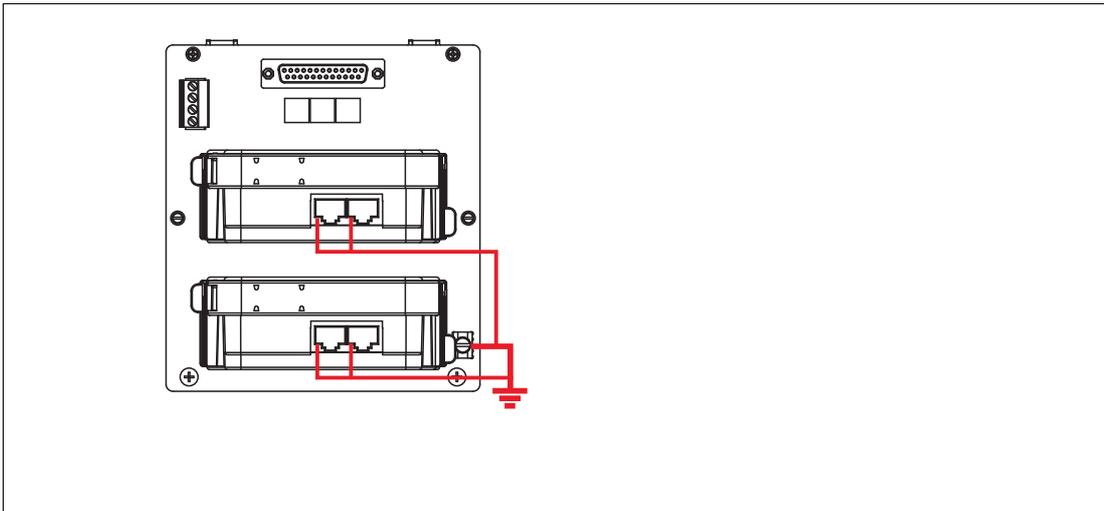
Figure 4.1 Stylized composition of the grounding
