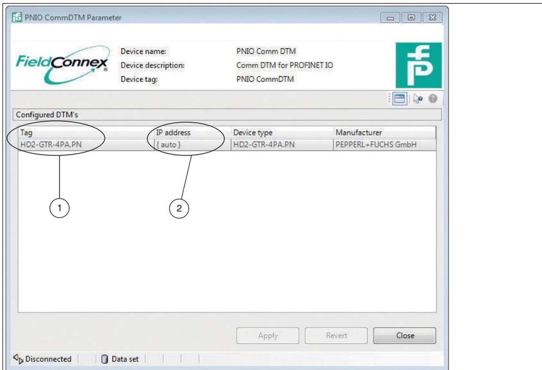
HD2-GTR-4PA.PN DTM configuration options for addressing the gateway
