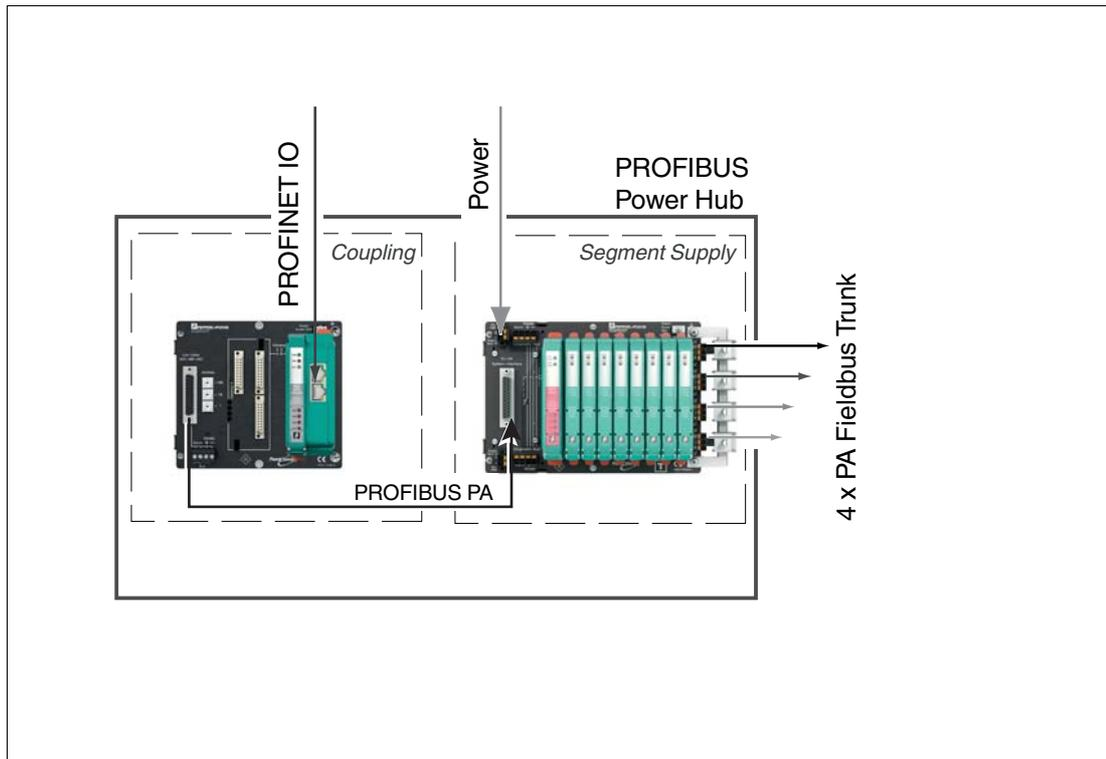
Figure 2.2 MBHC-FB-4R.HSC motherboard for the redundant supply of 4 segments combined with the MB-FB-GTR1 motherboard and 1 HD2-GTR-4PA.PN gateway module for gateway coupling.
