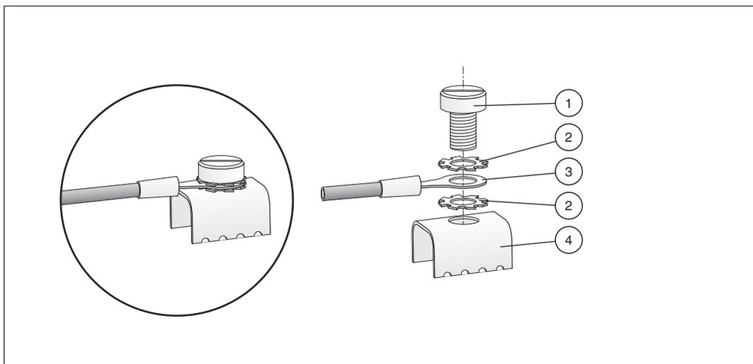
Figure 4.2 Connecting the ground connection cable
