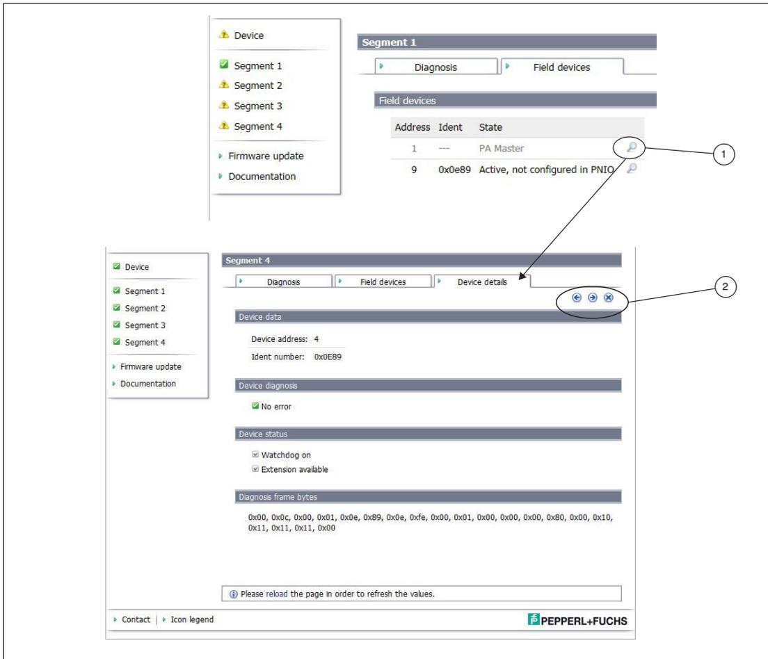
Figure 9.1 Web server user interface dialog **Segment 1 ... 4 > Field Devices**
