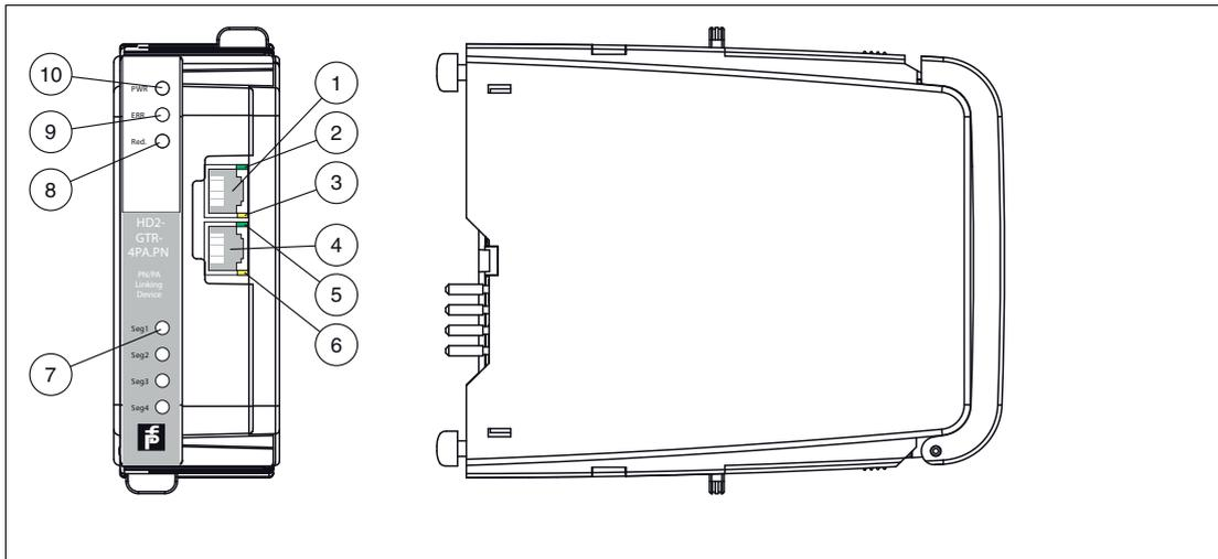
Figure 2.4 HD2-GTR-4PA.PN component identity
