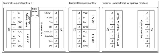
Figure 3.1 Terminal compartments
