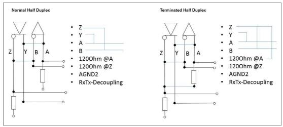
Figure 3.7 Half duplex cabling
