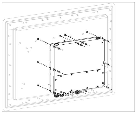
Figure 3.8 Mounting the TCU/PCU onto the display unit
