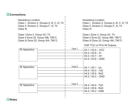
1. The Entity Concept allows interconnection of non-incendive apparatus with associated apparatus not specifically examined in combination as a system when the approved values of Voc (or Uo) and Isc (or Io) for the associated apparatus are less than or equal to Vmax (Ui) and Imax(Ii) for the non-incendive apparatus and the approved values of Ca(Co) and La(Lo) for the associated apparatus are greater than Ci + Ccable and Li + Lcable, respectively, for the non-incendive apparatus,
