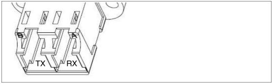
Figure 3.2 For the optional Fiber optic interface a duplex LC connection is required.
