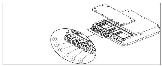
Figure 2.1 Cable gland connection layout
