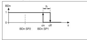
The switching signal is "active" (1), if the position value is smaller than the setpoint SP1. The value in SP2 is not used.
