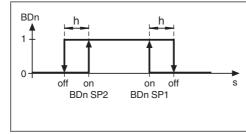
The switching system is "active" (1) if the position value is between setpoints SP1 and SP2. SP1 < SP2 does not invert the behavior.
