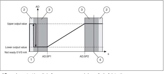
AO: analog output in volts/mA AD.SP1: position value range limit 1 AD.SP2: position value range limit 2
