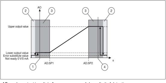
AO: analog output in volts/mA AD.SP1: position value range limit 1 AD.SP2: position value range limit 2 1: lower limit of detection range 2: no damping element detected 3: outside of the measuring range 4: upper limit of detection range
