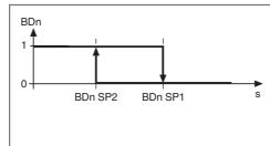
The switching signal is "active" (1) if the position value does not reach the lower setpoint SP2 and low "inactive" (0) if the position value exceeds the position value of setpoint SP1. SP1 < SP2 does not invert the behavior.
