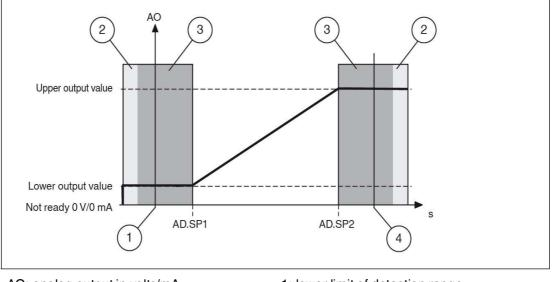
AO: analog output in volts/mA AD.SP1: position value range limit 1 AD.SP2: position value range limit 2
