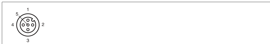
Figure 2.5 Schematic drawing of M12 socket, 5-pin, A-encoded, port X1 ... X8
