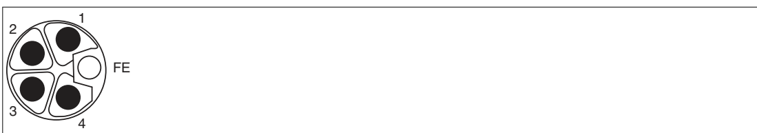
Figure 2.3 Schematic drawing of M12 L-encoding (plug); port X03 (IN)
