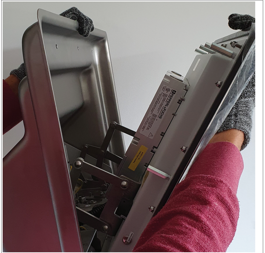
Figure 4.33 Display panel bolts lined up with the cutout holes of the housing.
