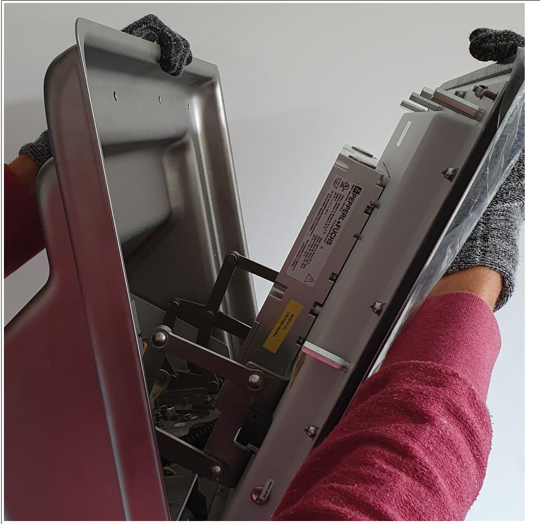
Figure 5.33 Display panel bolts lined up with the cutout holes of the housing.
