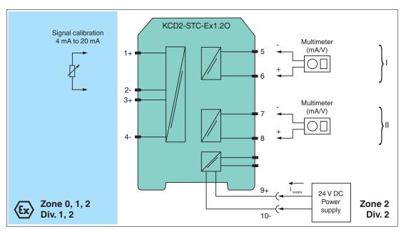
Figure 5.2 Proof test set-up for KCD2-STC-(Ex)1.2O.\*\*
