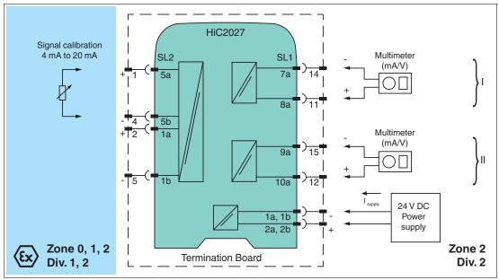
Figure 5.1 Proof test set-up for HiC2027\*\*
