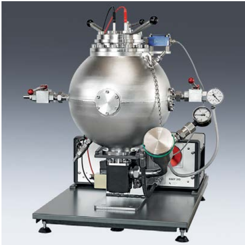
Figure 6. 20-L equipment for determining the rate of explosion pressure rise. Source: Kühne AG
