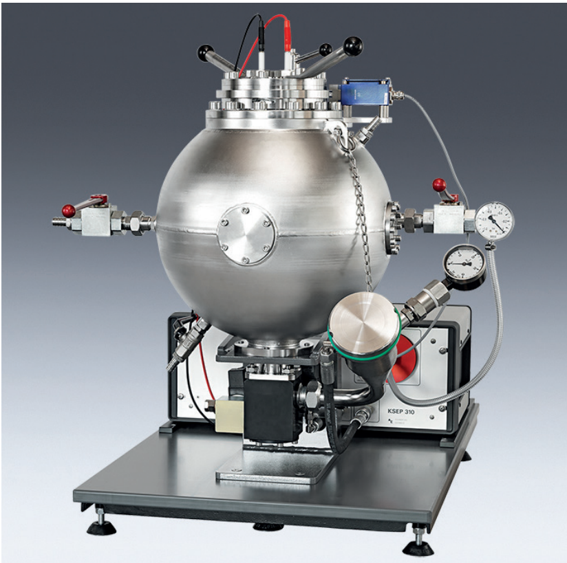
Figure 6. Equipment for determining the rate of explosion pressure rise Source: Kühne AG
