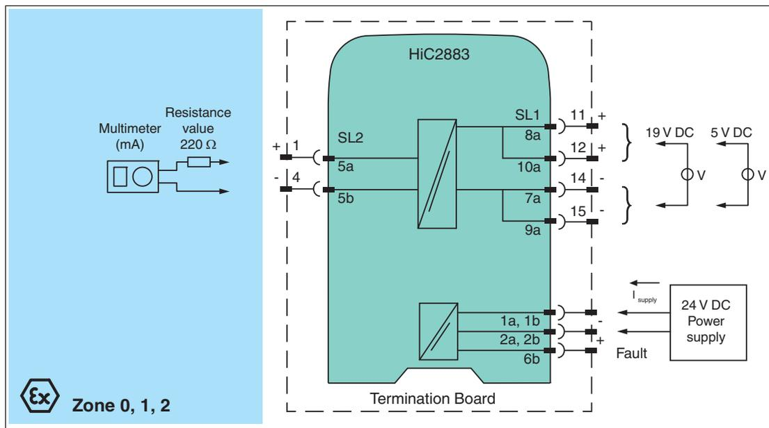
Figure 5.1 Proof test set-up for HiC2883
