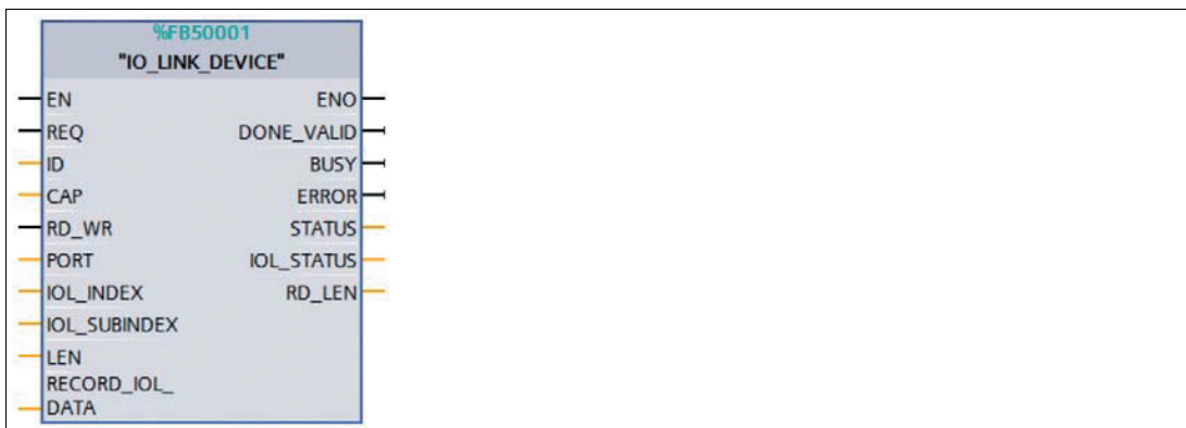
Figure 6.24 TIA Portal IO_LINK_DEVICE
