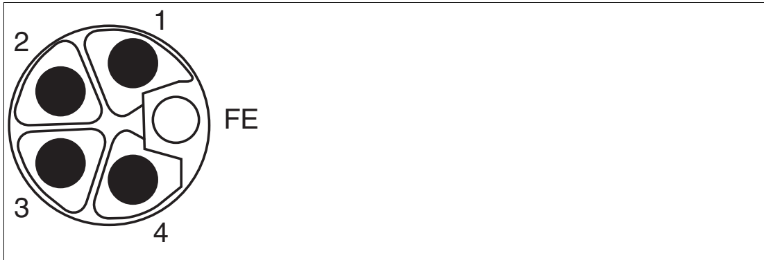
Figure 2.4 Schematic drawing of M12 L-encoding (plug); port X03 (IN)
