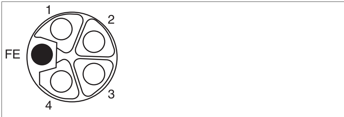
Figure 2.5 Schematic drawing of M12 L-encoding (socket); port X04 (OUT)
