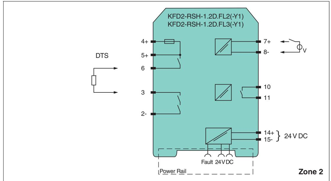
Figure 5.1 Standard application for dual pole switching
