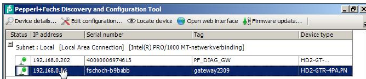
Figure 75: PROFINET gateway with the existing IP address
