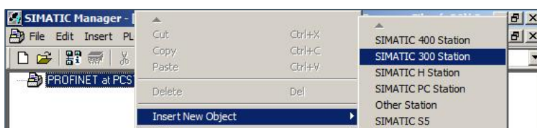
Figure 16: Choose the PCS model corresponding to the system hardware
