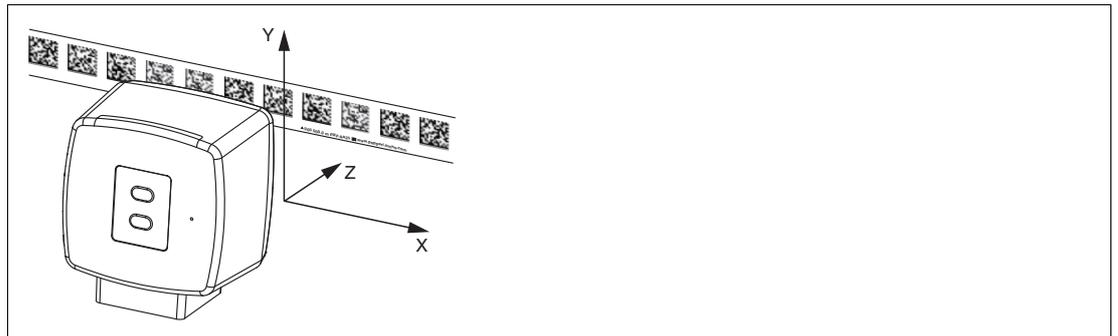
Figure 2.1 Schematic diagram of the alignment of the code tape and reader
