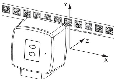
**Z coordinate:** If the distance between the camera and the code tape is too small, the yellow LED5 lights up. If the distance between the camera and the code tape is too large, the yellow LED5 goes out. Within the target range, the yellow LED5 and the green LED2 flash synchronously.
