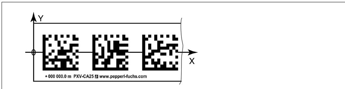
Figure 3.1 Zero line for code tapes
