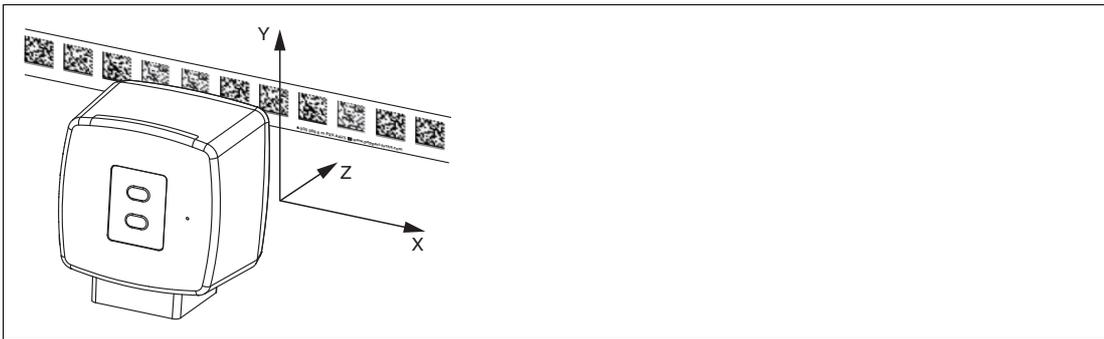
Position the code tape so that the **PEPPERL+FUCHS** logo and position markers are below the data matrix code. The position values then increase along the X direction. The diagram shows the orientation of a reader in the default setting of 0°. The reader can be configured in the interface for other installation situations.
