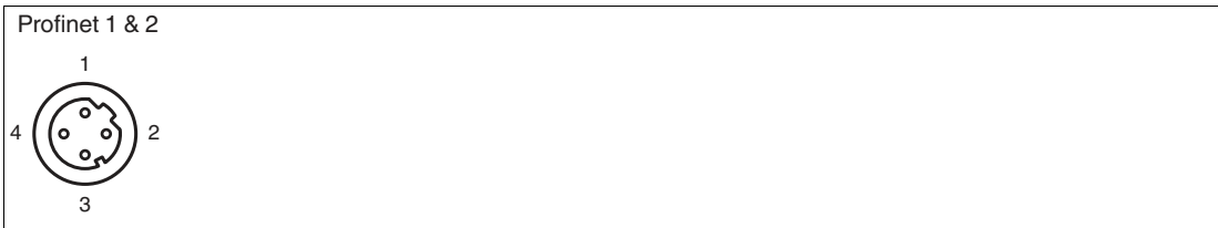
Figure 3.4 PROFINET connector assignment
