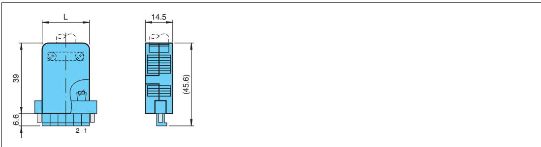
Figure 2.17 Dimensions of a cold junction with a protective cover L = 33.3 mm for 6-pin terminals
