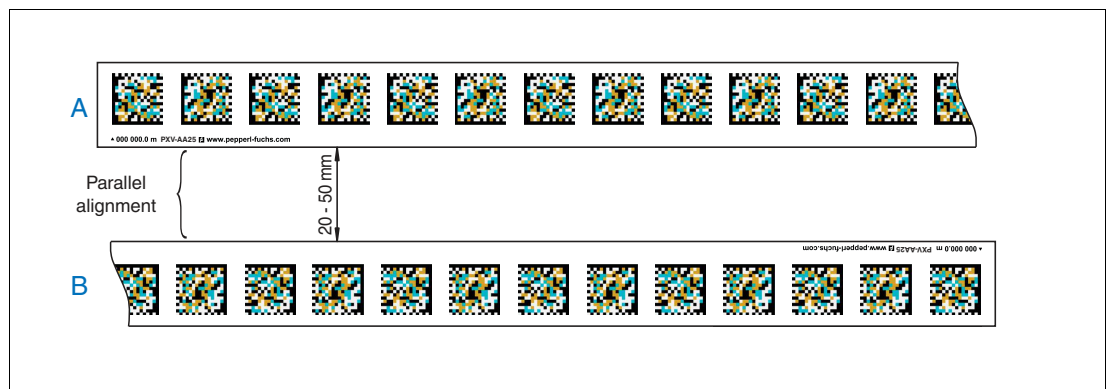
Figure 6.15 Schematic diagram: Reading behavior when changing lanes between 2 parallel Data Matrix code tapes. Possible distance between the Data Matrix code tapes: 20 mm ... 50 mm
