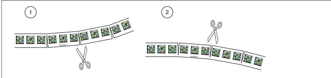
Figure 6.13 Schematic diagram: preparing Data Matrix code tape bends
