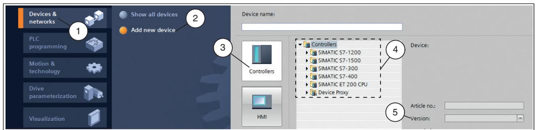
Figure 4.2 Adding a new device
