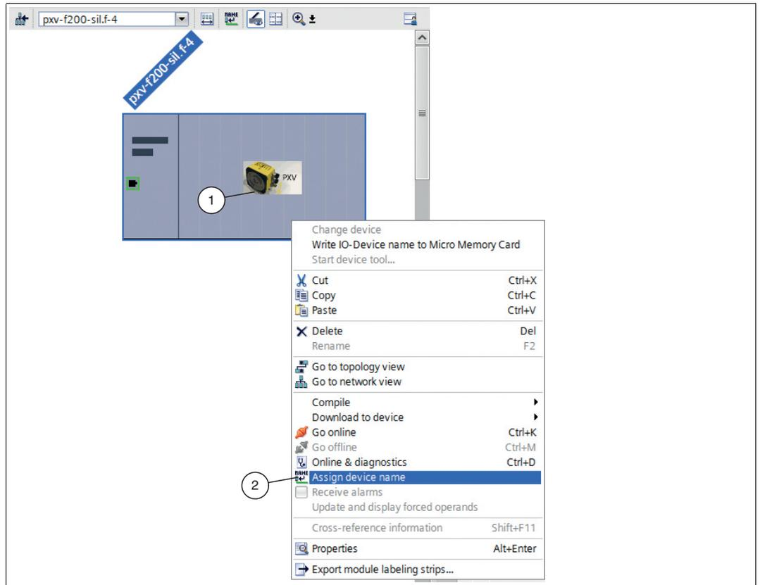
Figure 4.15 Assigning the device name
