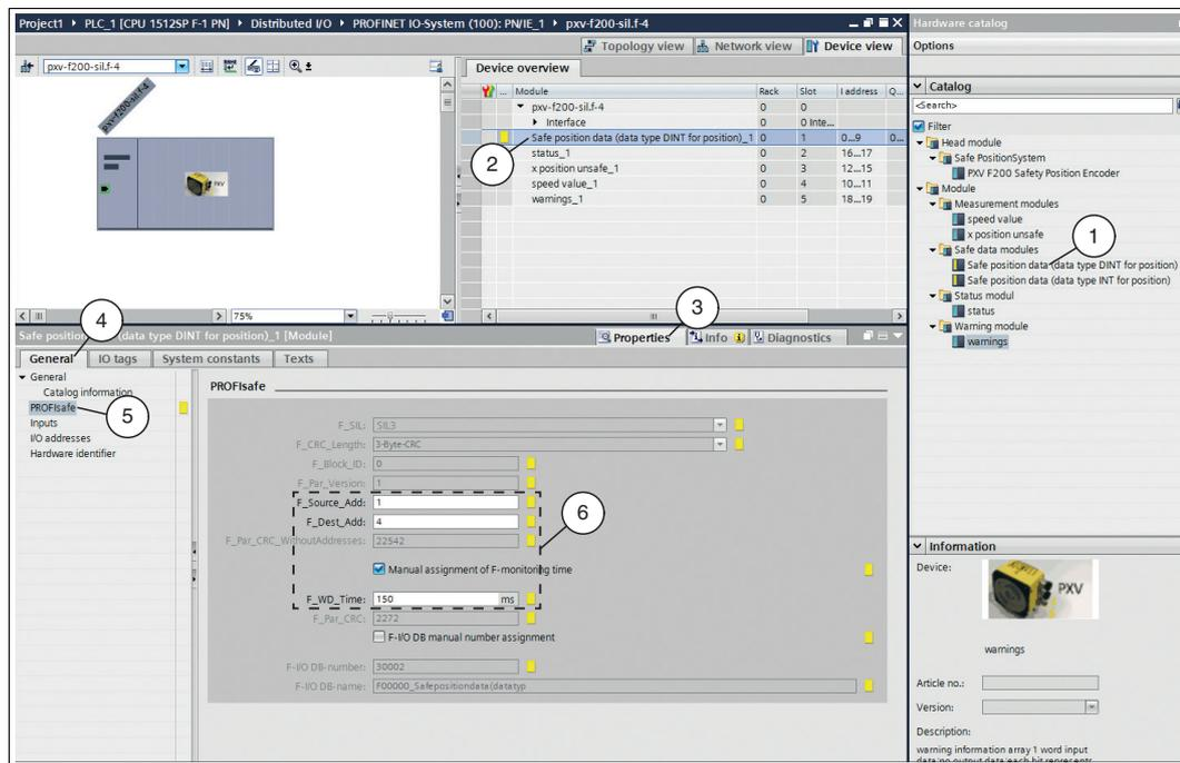
Figure 5.1 Configurable F-parameters
