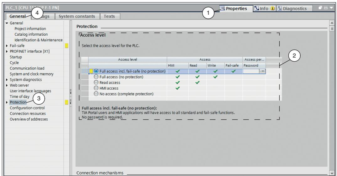
Figure 4.10 Control panel protection
