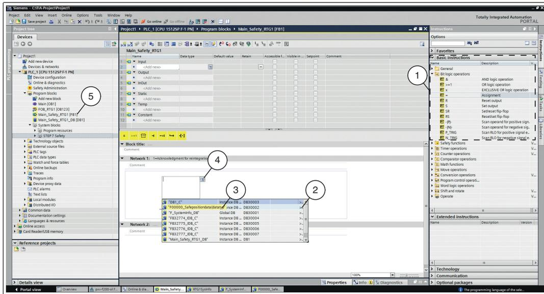
↳ In the work area, the program editor opens with the "Main\_safety\_RTG1 (FB1)" block. The right window range displays the list of all "Basic instructions" (1) that you need for programming.
