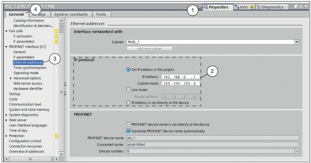
Figure 4.9 Ethernet address of the control panel
