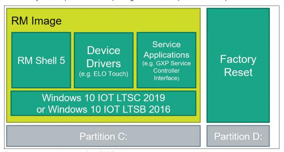
Figure 3.1 Architecture of the RM Shell
