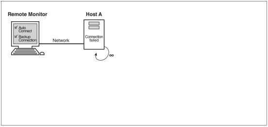
Figure 6.8 Example 1 - Unlimited number of retries to a specific host (with "Backup Connection" feature)
