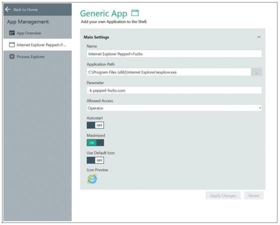
Figure 7.2 The "Generic App" window allows you to determine settings for new apps and adjust settings for existing apps.
