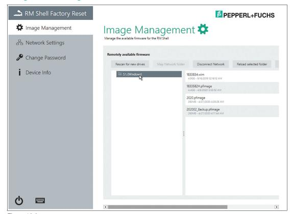
Figure 10.6 In this submenu you can manage the available firmware for the VisuNet RM Shell.
