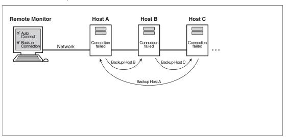
Figure 6.9 Example 2 - unlimited number of connection retries to more than one host (via "Backup Connection" feature)
