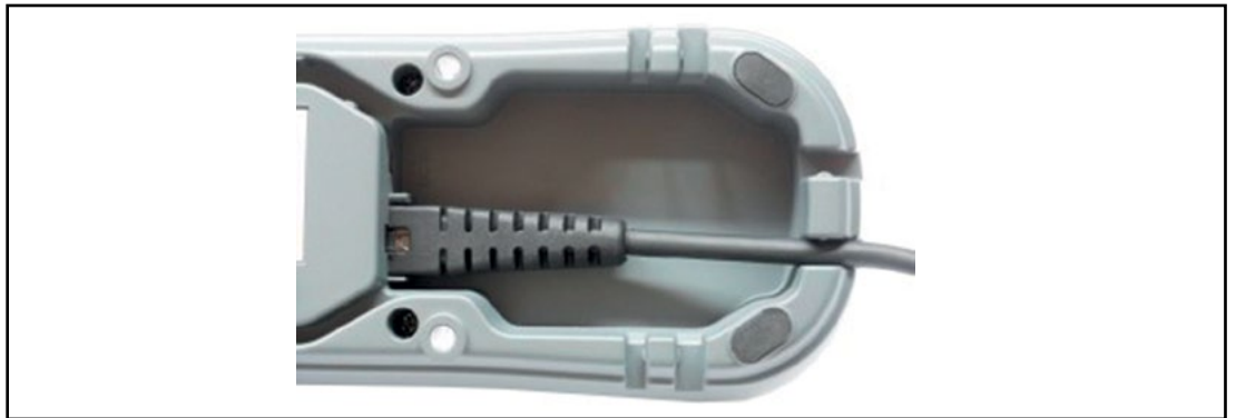
Figure 12. Connecting the RJ45 cable to the base station
