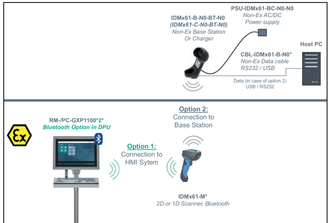
Figure 4. System structure 3—scanner with a base station in the safe area/Bluetooth option VisuNet GXP
