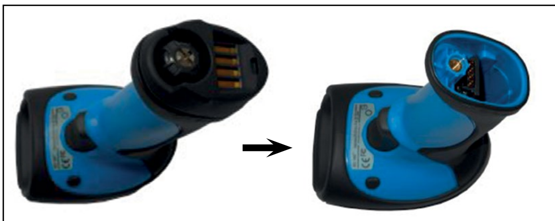
Figure 5. Removing the battery compartment lid
