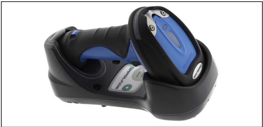
Figure 10. Inserting the scanner into the base station
