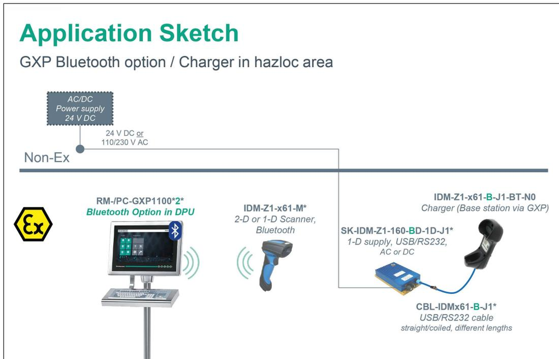
Figure 3.3 System structure 2 – scanner with base station connected to VisuNet GXP (Option 1)
