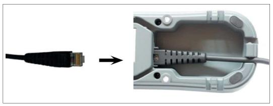
Figure 4.4 Connecting RJ50 connector of connection cable CBL-IDM\* to base station
