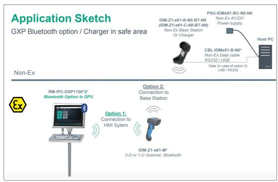
Figure 3.5 System structure 3 - scanner with a base station in the safe area/Bluetooth option VisuNet GXP
