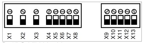
Figure 4.13 Terminal blocks in the terminal compartment
