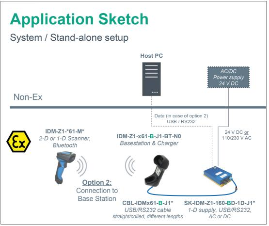
Figure 3.4 System structure 2 – scanner with base station connected to barrier (Option 2)
