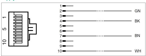
Figure 4.16 RJ50 plug - connection layout
