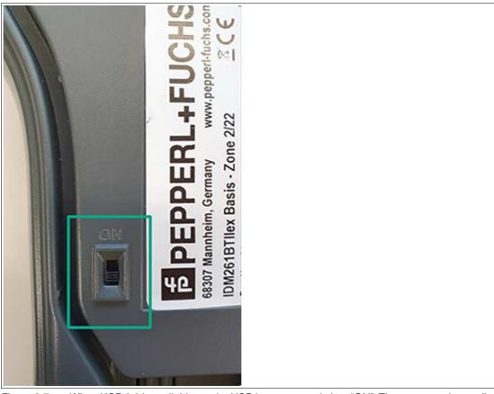
Figure 3.7 When USB 3.0 is available set the USB bus power switch to "ON". Then connect the cradle and host device via an USB cable.
