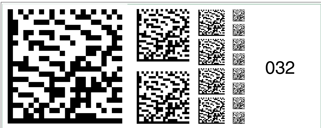
Figure 6.48 The code card "Fieldbus address 032" assigns the fieldbus address 032 to the device.
