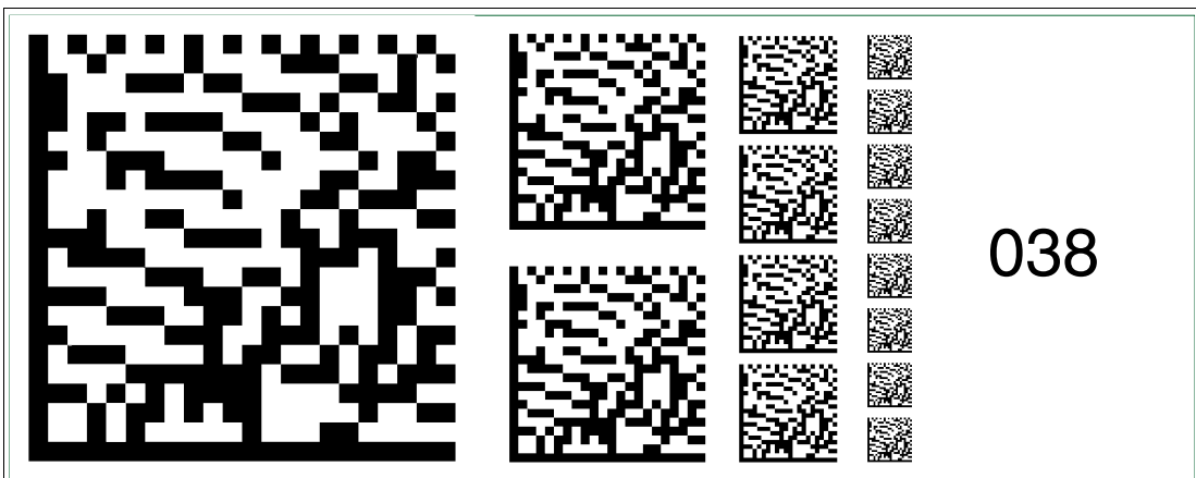
Figure 6.54 The code card "Fieldbus address 038" assigns the fieldbus address 038 to the device.
