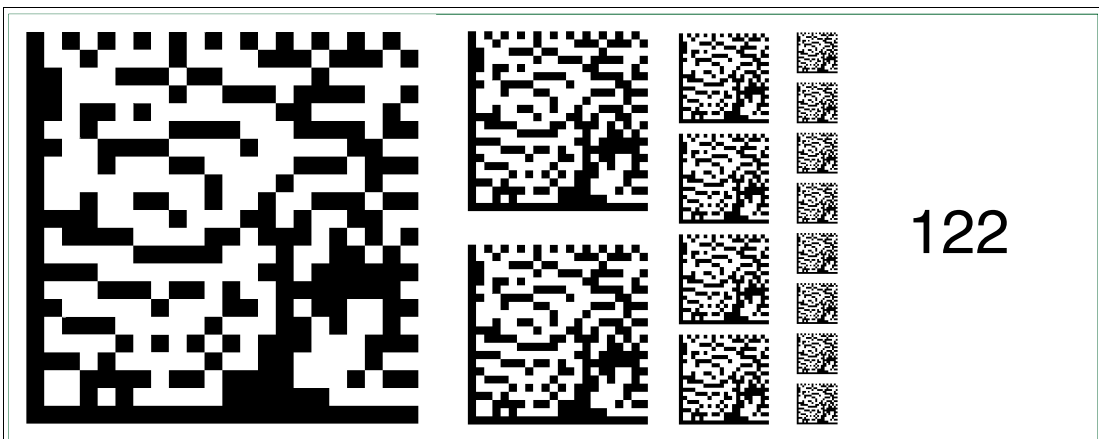
Figure 6.138 The code card "Fieldbus address 122" assigns the fieldbus address 122 to the device.
