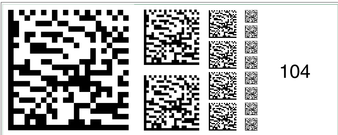
Figure 6.120 The code card "Fieldbus address 104" assigns the fieldbus address 104 to the device.
