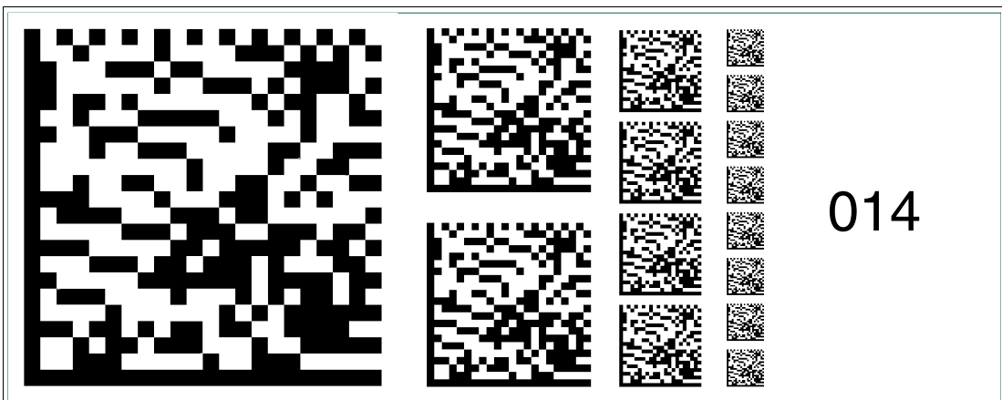
Figure 6.30 The code card "Fieldbus address 014" assigns the fieldbus address 014 to the device.
