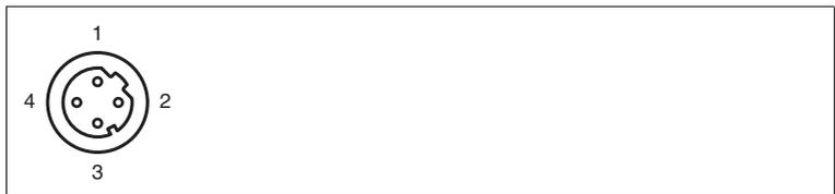
Figure 3.3 Ethernet connection layout
