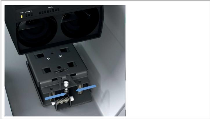
5. Click the device into the openings. Make sure that the retaining feet of the device are engaged far enough that you can push the two latches outward fully. To do this, push in the center of the device, applying some force from above if necessary.
