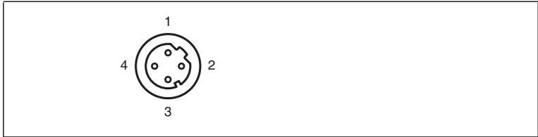
Figure 3.2 Connection layout for network socket
