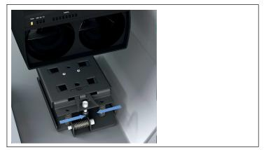
Click the device into the openings. Make sure that the retaining feet of the device are engaged far enough that you can push the two latches outward fully. To do this, push in the center of the device, applying some force from above if necessary.
