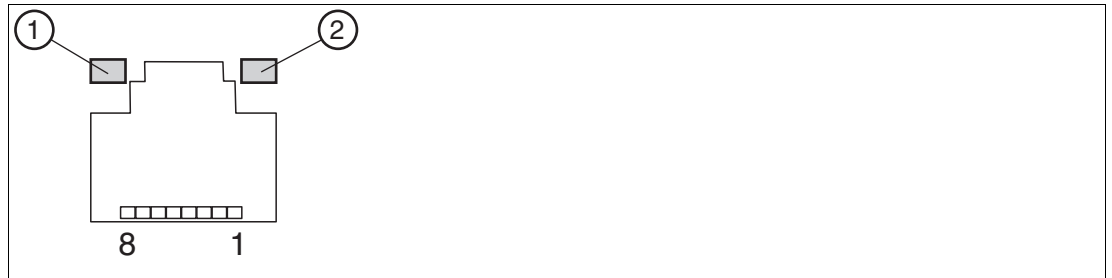
Figure 4.18 RJ45 pinout with LED display
