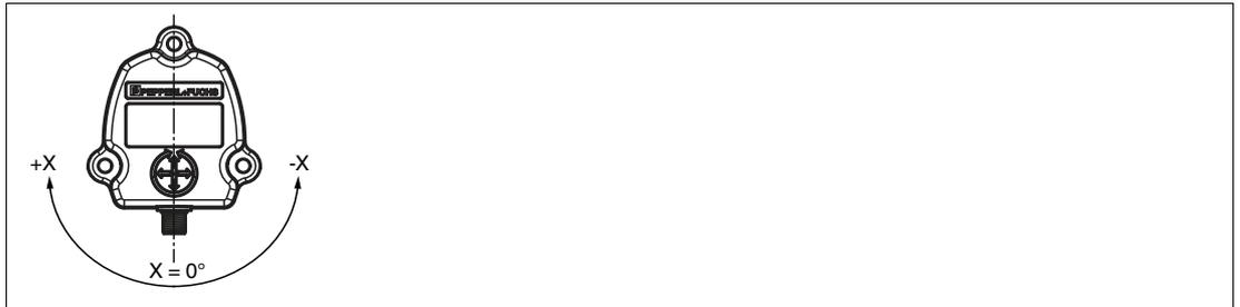
Figure 3.1 1-axis sensor
