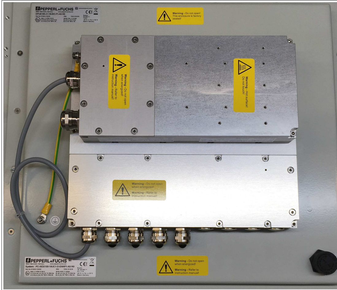
Figure 3.9 Factory-assembled ground connection from PSU to DPU
