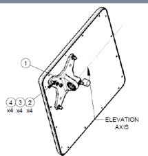
Attach item 1 to the back of the antenna using items 2, 3, 4 as shown.
