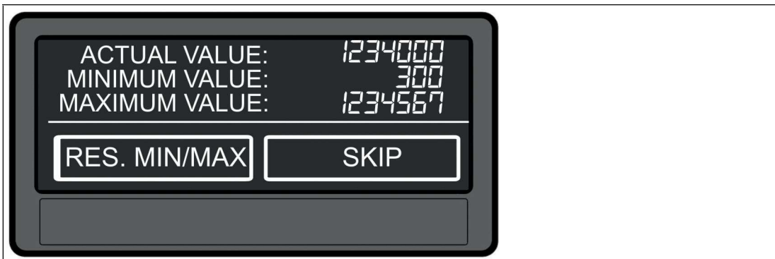
Figure 4.9 Tap the top of the touch screen or press Skip to change to the next display.
