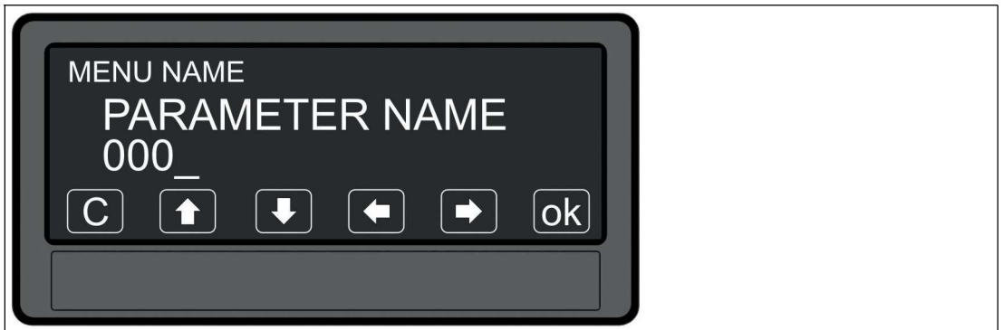
Figure 4.4 Use the arrow keys to edit the selected parameter and save by pressing "OK." Pressing "C" exits the editing screen.
