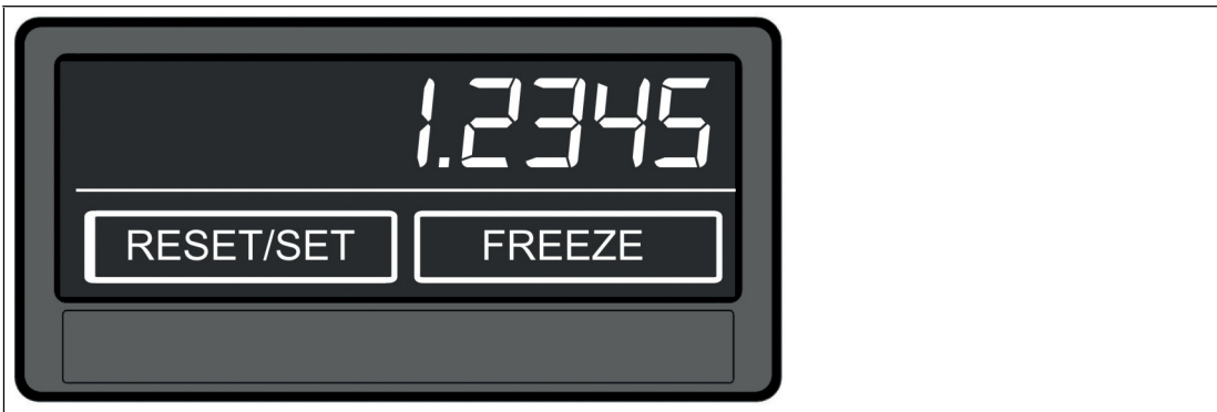
Figure 4.7 Tap the top of the touch screen to change to the next display. Only enabled in TIMER or COUNTER mode.
