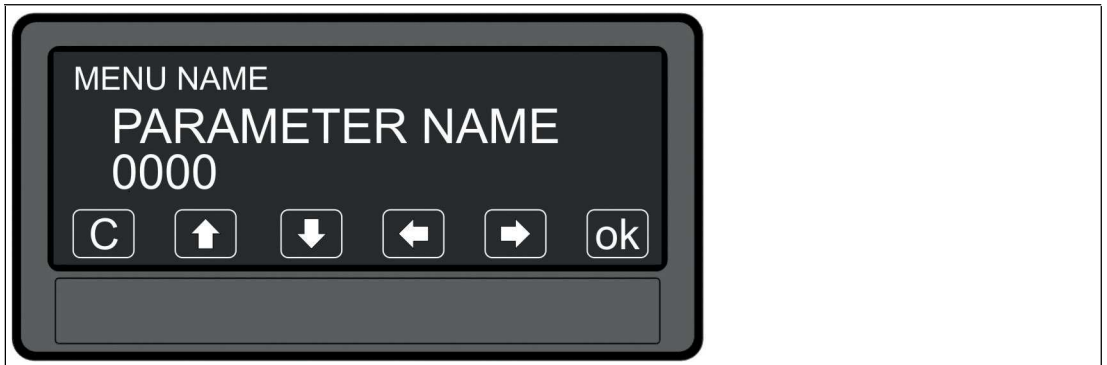
Figure 4.3 Use the arrow keys to select the required parameter and confirm by pressing "OK." Pressing "C" exits the parameter selection.
