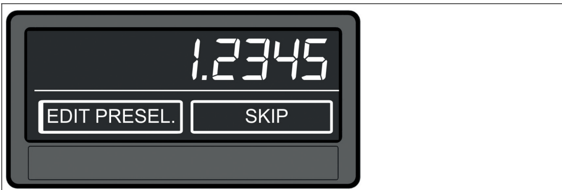
Figure 4.8 Tap the top of the touch screen or tap Skip to change to the next display.
