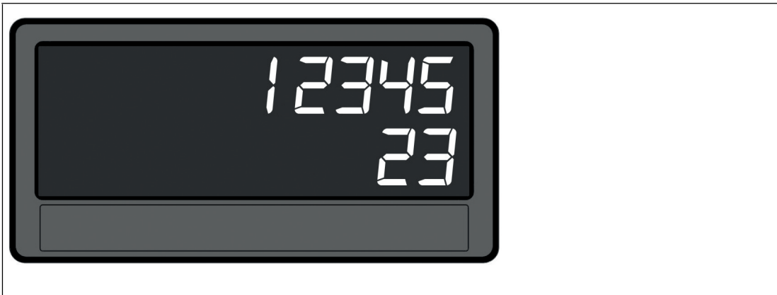
Figure 4.6 Tap the top of the touch screen to change to the next display. Only enabled in COUNTER - BATCH MODE.
