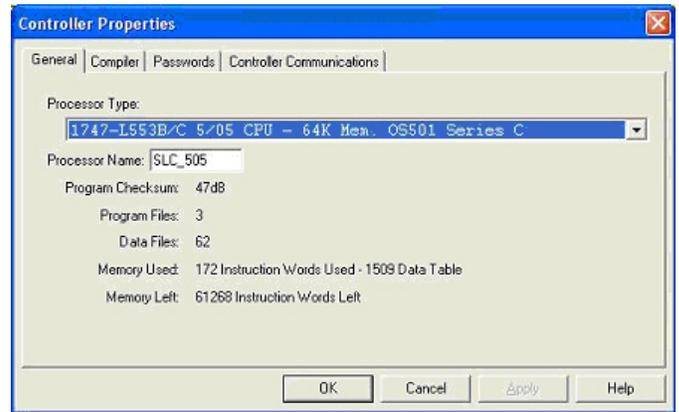
3. Select the **Controller Communications** tab and select the proper driver for RSLogix 500.
