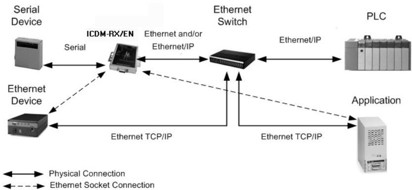
EtherNet/IP firmware provides an application interface for both serial and Ethernet devices. You can connect any application, such as a configuration, database, or control application, via the application socket port to the serial and/or Ethernet devices while the device(s) are attached to the PLC via EtherNet/IP.
