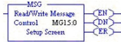
1. Assign a dedicated message file to the **Control** block in the ladder logic (as shown above).
