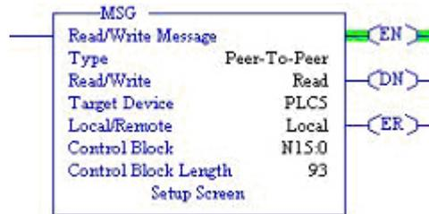
In the ladder logic, double-click the **Setup Screen** in the **MSG** instruction.
