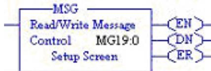
1. Assign a dedicated message file to the **Control** block in the ladder logic (as shown above).
