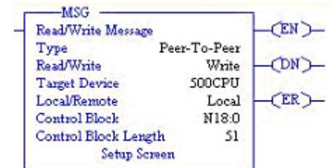
5. In the ladder logic, double-click the **Setup Screen** in the **MSG** instruction.
