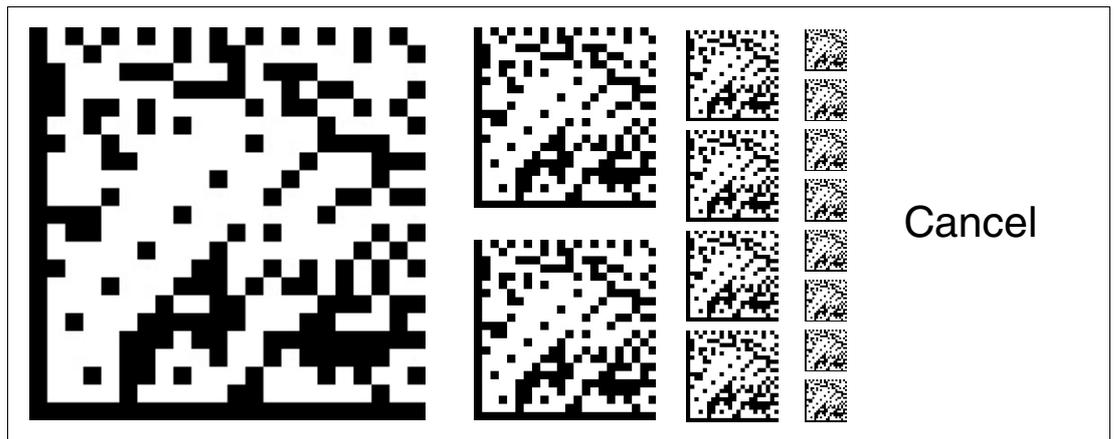
Figure 6.4 The "CANCEL" code card discards the modified parameterization and terminates external parameterization operating mode. The read head switches to normal mode and adopts the last valid configuration that was saved.
