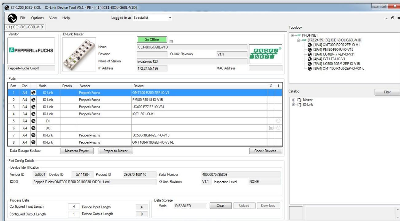
Configuration tool with IO-Link of a device and the device information it contains
