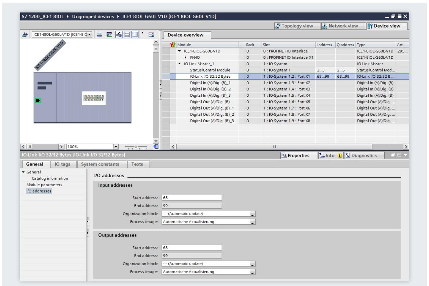
A screenshot of the STEP 7 TIA Portal software interface showing the 'Device overview' and 'I/O addresses' configuration for an IO-Link master module. The window title is 'S7-1200\_ICE1-8IOL > Ungrouped devices > ICE1-8IOL-G60L-V1D [ICE1-8IOL-G60L-V1D]'. The 'Device overview' table lists the module and its properties. The 'I/O addresses' section shows the input and output address ranges for the IO-Link master.
