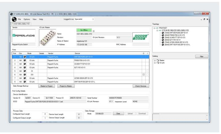
Configuration tool with IODD of a device and the device information it contains
