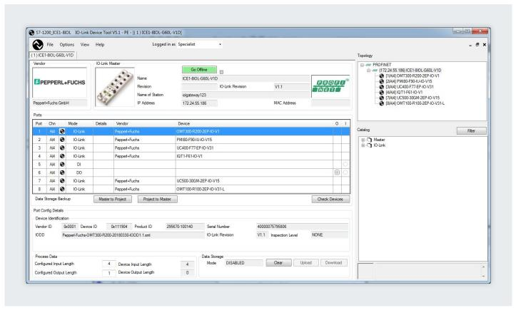
Configuration of an IO-Link master in the configuration tool
