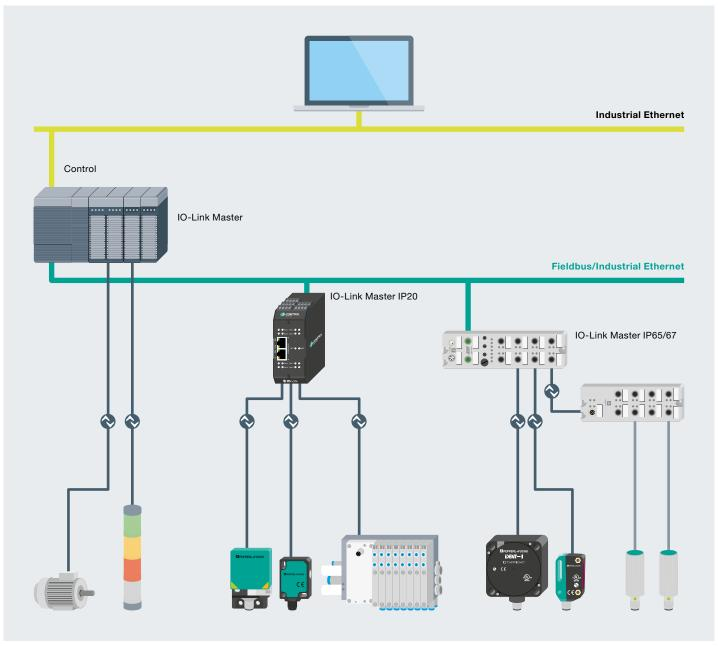
Example of a system architecture with IO-Link.
