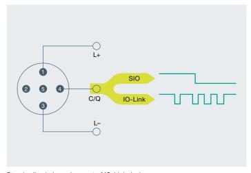
Standardized pin assignment of IO-Link devices
