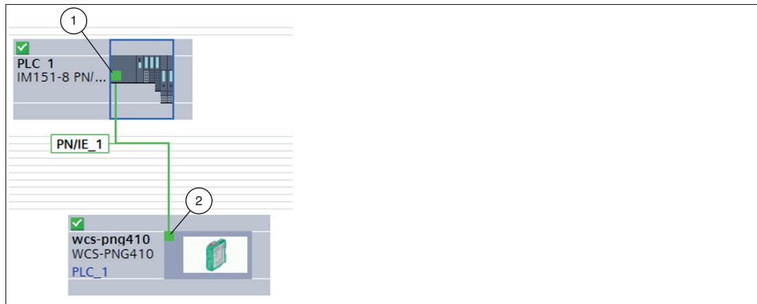
Figure 4.10 Connecting the interface module to the control panel
