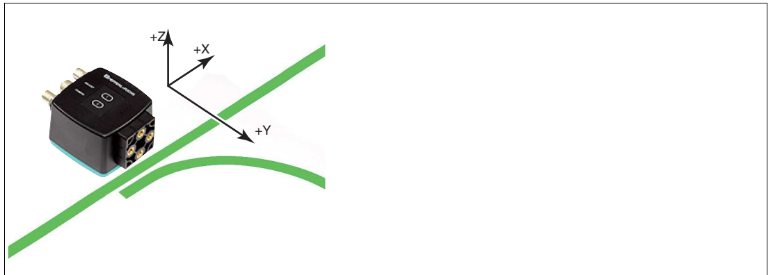
Figure 3.2 Field of view and coordinates of the sensor
