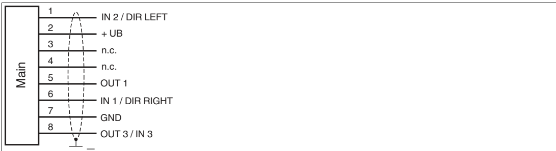
Figure 3.22 Electrical connection of the read head
