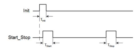
T:  $1 \mu s \dots 9 \mu s$  (adjustable)
