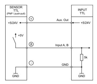
In general, open PNP inputs are "LOW" and open NPN inputs are "HIGH."
