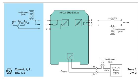
Figure 5.1 Proof test set-up for KFD2-SR2-Ex1.W
