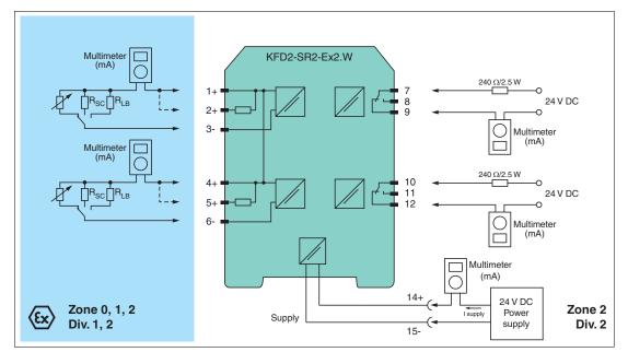
Figure 5.3 Proof test set-up for KFD2-SR2-Ex2.W
