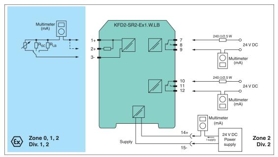
Figure 5.2 Proof test set-up for KFD2-SR2-Ex1.W.LB
