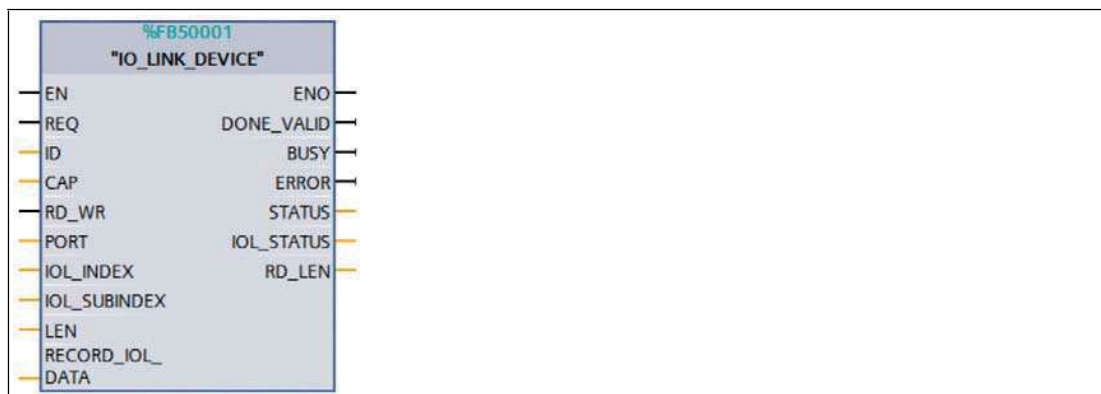
Figure 5.22 TIA Portal IO_LINK_DEVICE
