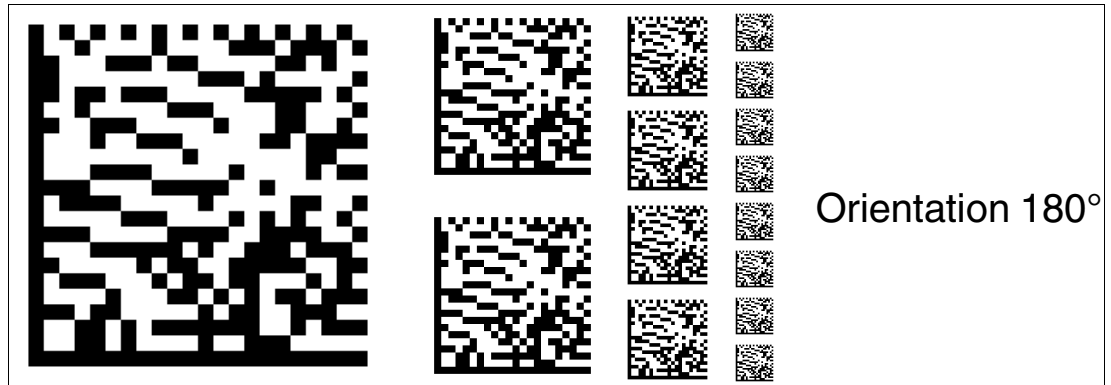
Figure 6.10 The code card assigns the orientation 180° to the read head.
