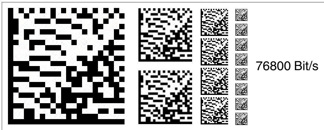
Figure 6.14 The transfer rate of the read head for communication via the interface is preset to 76800 bit/s.
