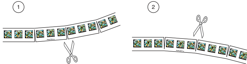
Figure 3.1 Schematic diagram: preparing Data Matrix code tape bends
