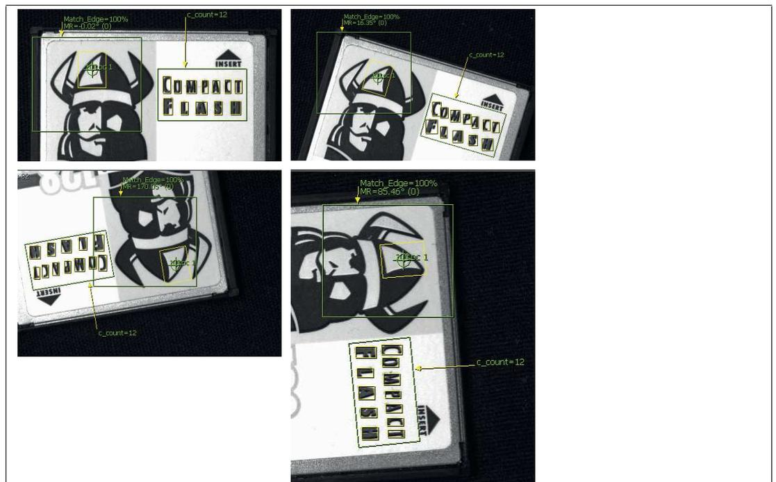
Figure 7.11 Example: edge-based object comparison
