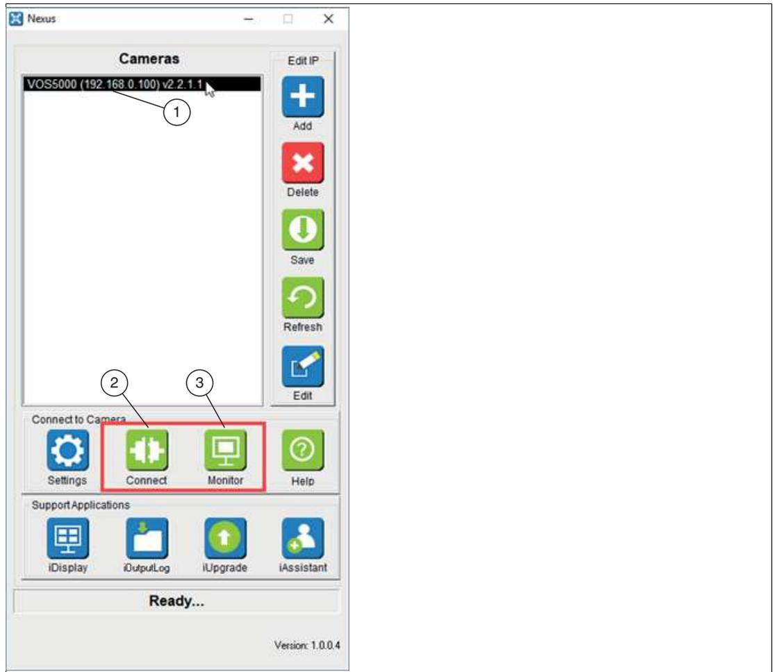
Figure 6.10 Establishing a sensor connection
