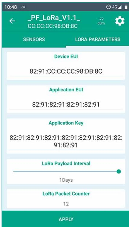
With WILSEN.sonic.level, you can access this 16-digit Device EUI in hexadecimal format by connecting to the device via the WILSENcontrol app (see brief commissioning instructions). The device-specific *Device EUI* is displayed under the *LORA PARAMETERS* tab in the app.
