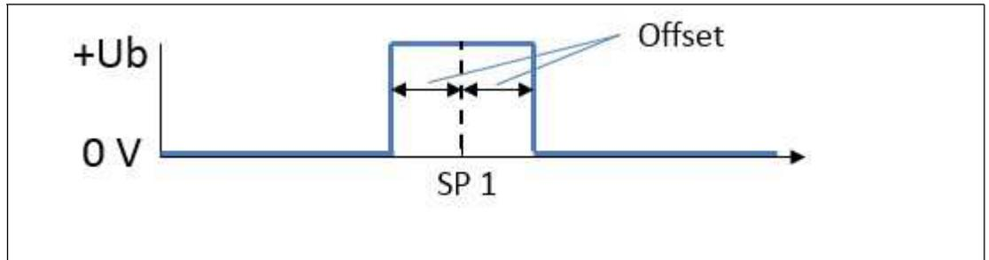
Figure 8.4 Example of behavior of a "normally-open" push-pull / PNP switching output in retroreflective mode
