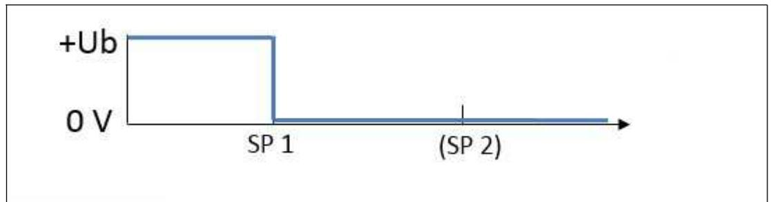
Figure 8.1 Example of behavior of a "normally-open" push-pull / PNP switching output in switch point mode
