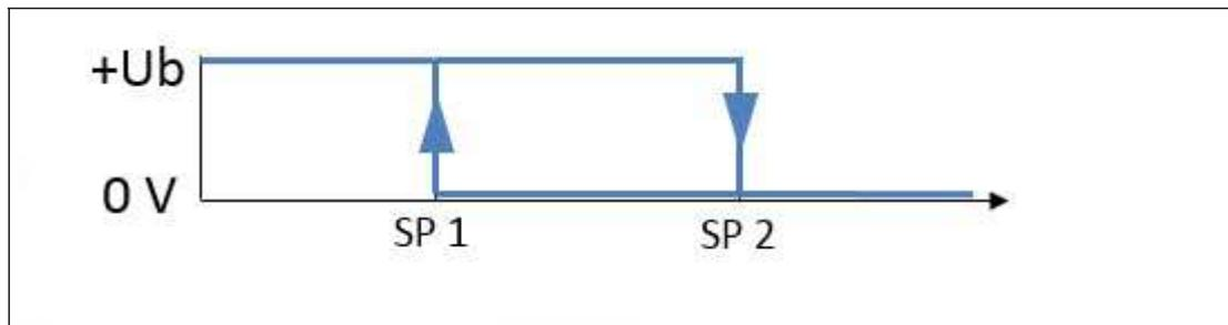
Figure 8.3 Example of behavior of a "normally-open" push-pull / PNP switching output in hysteresis mode
