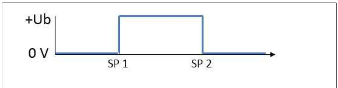
Figure 8.2 Example of behavior of a "normally-open" push-pull / PNP switching output in window mode
