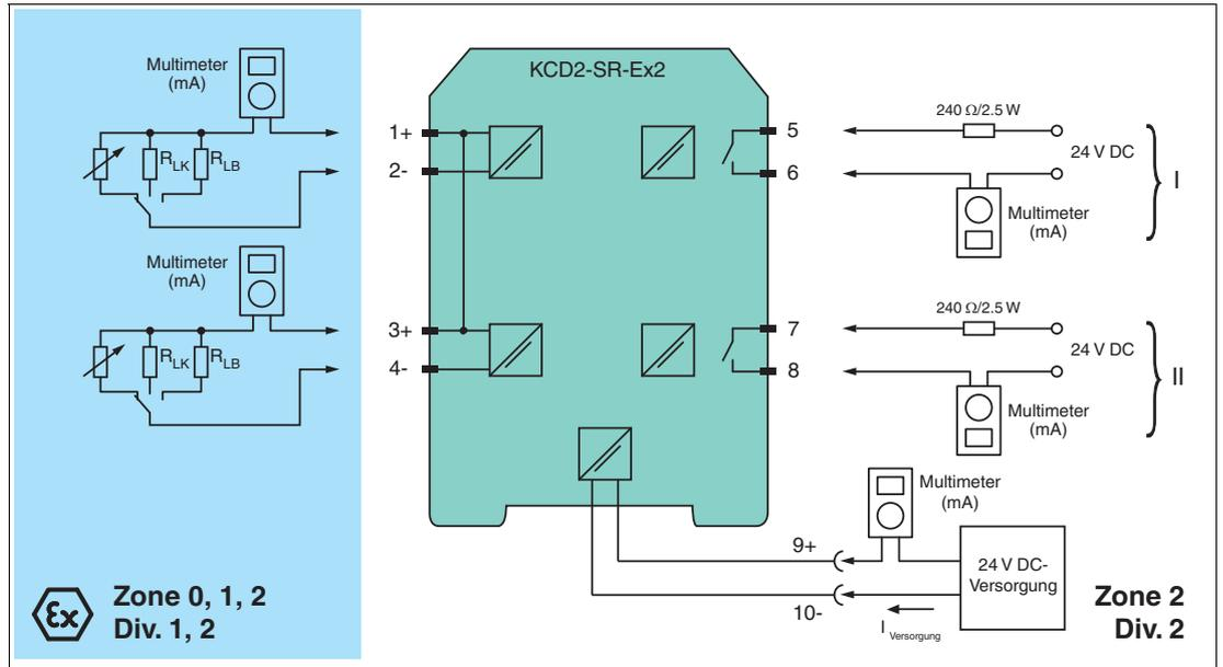
Figure 5.3 Proof test set-up for KCD2-SR-(Ex)2(.SP)
