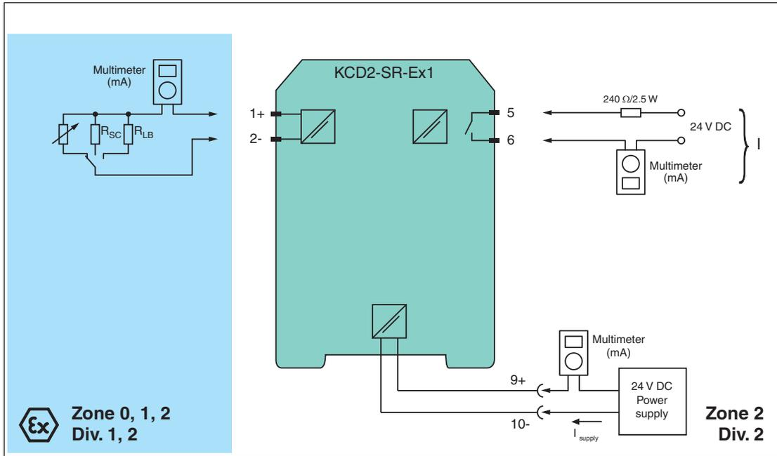
Figure 5.1 Proof test set-up for KCD2-SR-(Ex)1
