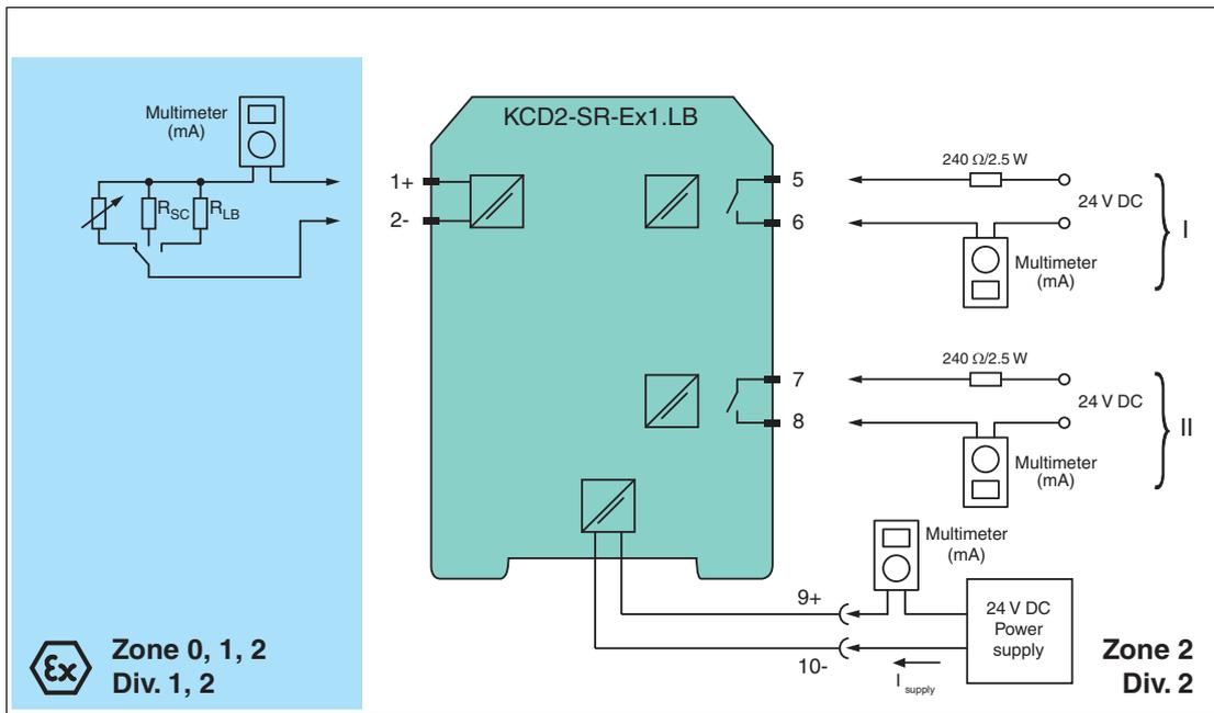
Figure 5.2 Proof test set-up for KCD2-SR-(Ex)1.LB(.SP)
