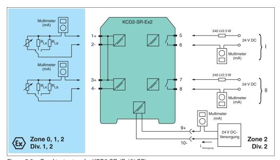
Figure 5.3 Proof test set-up for KCD2-SR-(Ex)2(.SP)
