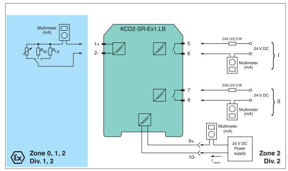
Figure 5.2 Proof test set-up for KCD2-SR-(Ex)1.LB(.SP)
