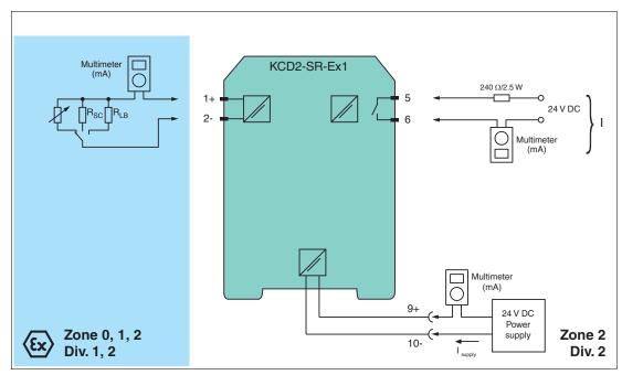
Figure 5.1 Proof test set-up for KCD2-SR-(Ex)1
